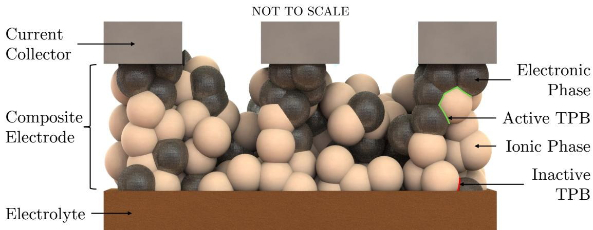
Figure 1.1: Model of a composite porous SOFC electrode, highlighting phase composition and TPB activity.
